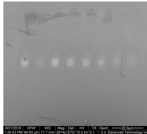
SEM image of eight regions implanted with Ge/25 keV over a range of fluences between 1 \times 10^{17}/\text{cm}^2 to 4 \times 10^{16}/\text{cm}^2 post-anneal and Al removal.
